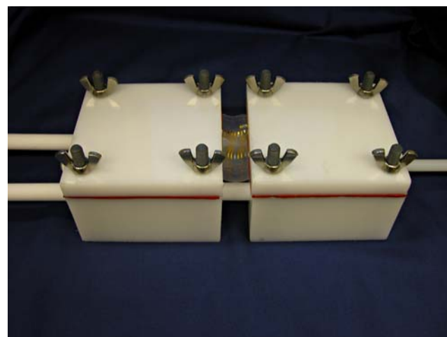
Fig. 6 Uniaxial strain device for electro-mechanical evaluation of the PDMS-based MEA. The custom-made apparatus shown was used to clamp the MEAs and apply uniaxial strain in 1% increments
