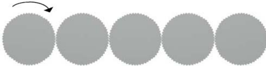
Figure 3. Series of gears in which the first turns clockwise. In which direction will the last gear turn?
